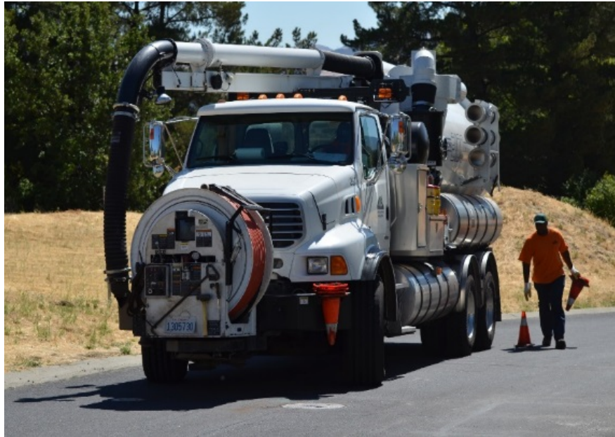
Figure 4.3 Central San Hydroflush Truck
