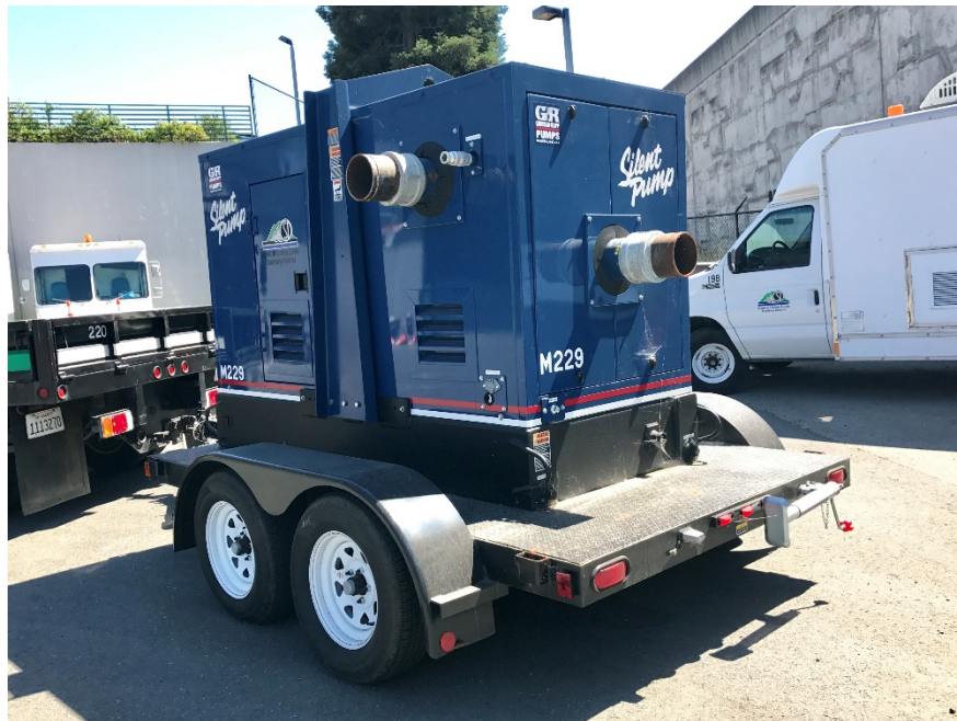
Figure 4.18 Gorman-Rupp Bypass Pump at CSO
