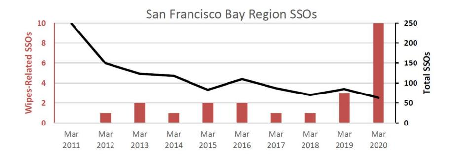
**\*SSO = Sanitary Sewer Overflow.** This means that something (in this case, wipes) was blocking wastewaters' movement through pipes underneath the ground. The result was a sewer overflow.
